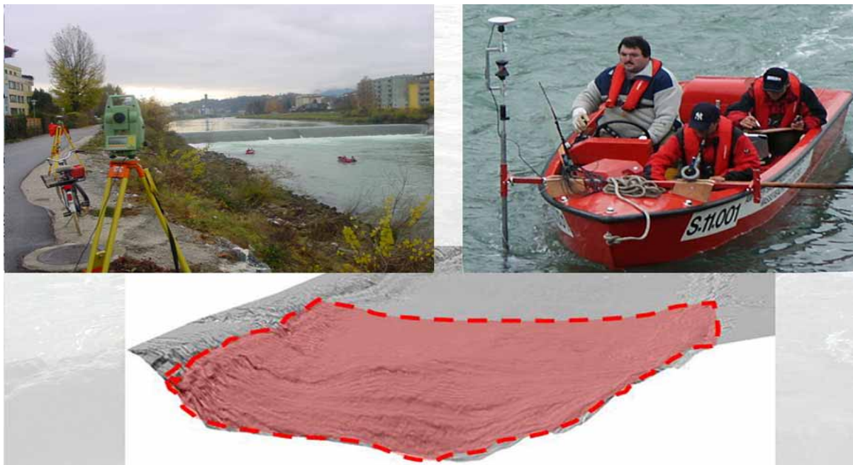
Fig.7: Application of the coupled GPS/TPS positioning unit for measuring the stilling basin in the city of Salzburg and resulting digital terrain model of the basin floor
