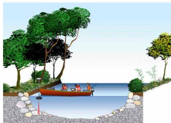
Fig.3: Scheme of a typical profile measuring operation
