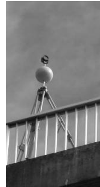
Fig. 9: Target spheres for short range and long range measurements: Diameters, 76.2mm and 239.7mm, respectively
