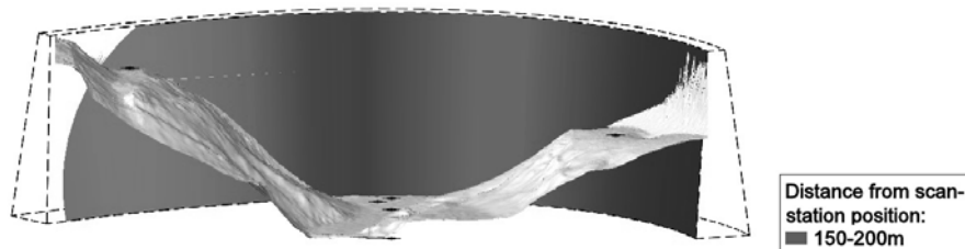
Fig. 5: Simulation of scan ranges; standard mounting of the scanner; axis not tilt → scan ranges between 160 m and 240 m
